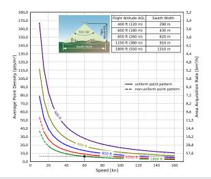
Example: VUX-160 $^{23}$  at 300,000 pulses/sec, laser power level 100% altitude 1,800 ft AGL, speed 60 kn, resulting point density  $\sim6.2$  pts/m $^2$
