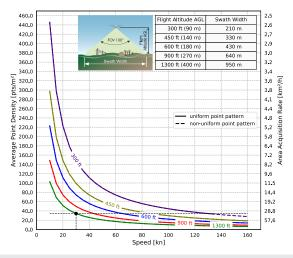
Example: VUX-160 $^{23}$  at 600,000 pulses/sec, laser power level 100% altitude 1,300 ft AGL, speed 30 kn, resulting point density  $\sim 34$  pts/m $^2$
