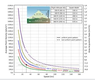
Example: VUX- $160^{23}$  at 1,800,000 pulses/sec, laser power level 100% altitude 550 ft AGL, speed 30 kn, resulting point density  $\sim 243$  pts/m<sup>2</sup>
